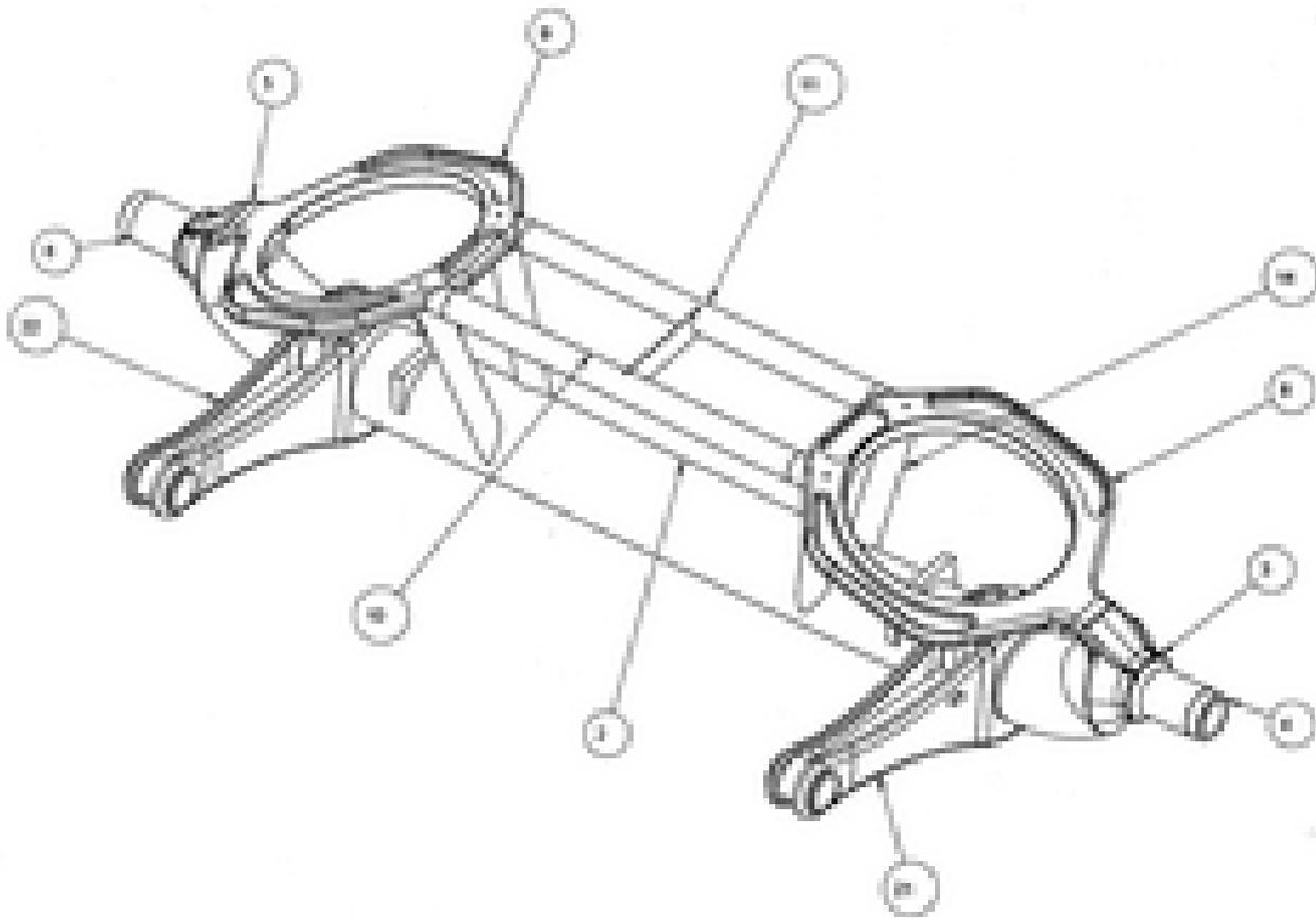
Presented here is a rigid, non-driven lightweight chassis for utility vehicles that offers a significant weight advantage and improved suspension properties. In addition it includes a build-in mechanism for cost-effective wheel alignment.
