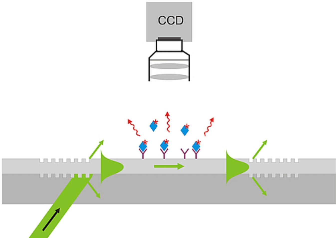
*Figure 1: Function principle of evanescent field microscopy: The light of a laser is coupled into a microscope slide via a grating structure. The evanescent field stimulates optical transitions in molecules located on the surface of this carrier. (Source: Fricke-Begemann)*
