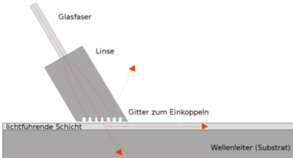
*Figure 2: Functionality of the simplified structure: The light is guided via a glass fibre to a lens. This is ground on the side facing the waveguide and provided with a grating. This means that the grating no longer has to be applied to the light-conducting layer of the waveguide. If there is sufficient proximity between the grating and the waveguide, the laser light is coupled in. (Source: Fricke-Begemann)*
