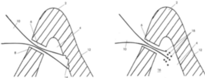
*Laser drilling without backing material damages the workpiece. A nanoparticle-suspension helps to prevent the damage. (Source: Patent application DE102013212665B4)*
