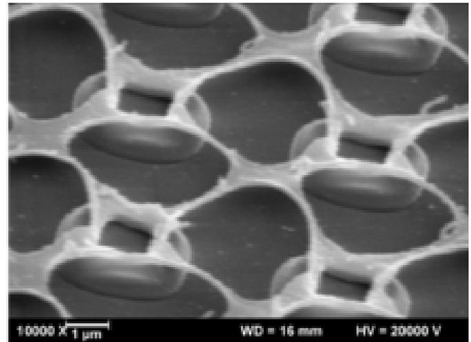
*Example of a net-like surface with periodic structures under two different angles. At locations that have been irradiated with lower laser intensity, the structure stays bonded to the substrate while at locations of high laser intensity it is burst open and separated. For the shown structure, the period length is approximately five micrometers. (Source: Weichenhain-Schriever, Ihlemann)*
